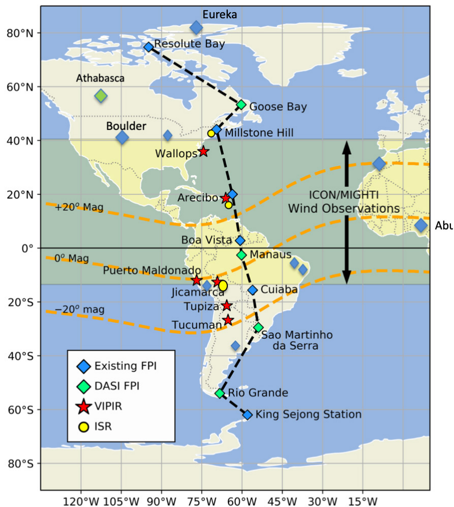
Figure 24: A proposed expansion plan for the Fabry-Perot Interferometer network in the American sector called Distributed Array of Small Instruments (DASI). If IMCP can provide infrastructure at locations like Goose Bay, Rio Grande, and others, we will have a complete chain. The geographical coverage of the ICON/MIGHTI wind observations is also indicated.
